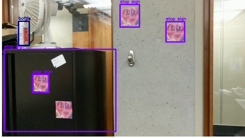
Figure 6: Sample frame from our creation attack video after being processed by YOLO v2. The scene includes 4 adversarial stickers reliably recognized as Stop signs.
